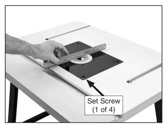
Figure 14. Using the straightedge on the mounting board and table.
